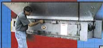
1 Screen Access Via Hinged Door
