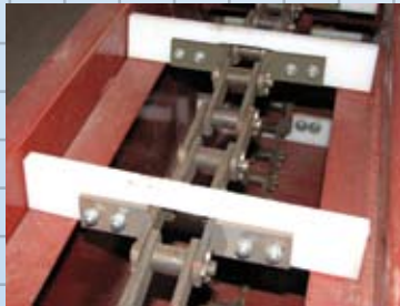
(Left) Chain cleaner shown in conveyor trough before chain is installed. The cleaner pivots down to clean the chain when discharge is at that gate, or pivots up and out of the way when material is going past that gate to another one. (Center) conveyor section with cover removed for photo. Fertilizer is carried "en masse" in a much deeper pile than the height of the flights. Chain returns on top side, riding on stainless return rails. (Right) Model 1211 En Masse conveying DAP fertilizer.
