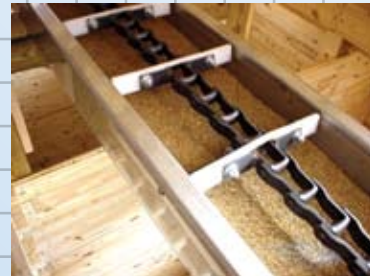
(Left) Chain cleaner shown in conveyor trough before chain is installed. The cleaner pivots down to clean the chain when discharge is at that gate, or pivots up and out of the way when material is going past that gate to another one. (Center) conveyor section with cover removed for photo. Fertilizer is carried "en masse" in a much deeper pile than the height of the flights. Chain returns on top side, riding on stainless return rails. (Right) Model 1211 En Masse conveying DAP fertilizer.
