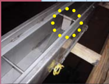
(Left) Chain cleaner shown in conveyor trough before chain is installed. The cleaner pivots down to clean the chain when discharge is at that gate, or pivots up and out of the way when material is going past that gate to another one. (Center) conveyor section with cover removed for photo. Fertilizer is carried "en masse" in a much deeper pile than the height of the flights. Chain returns on top side, riding on stainless return rails. (Right) Model 1211 En Masse conveying DAP fertilizer.
