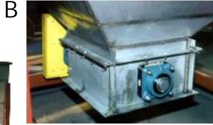
A- 6' X 6' hopper mounted over model 21 Lump-Buster B- Note waste pack seal for bearing protection C- Payloader style hopper over Lump-Buster. Note grate. E- Model 21 showing standard Drive package for models 21-90
