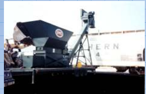
Model 90 Lump-Buster with 12' X 5' payloader hopper, Mounted over Bulk-Toter.
