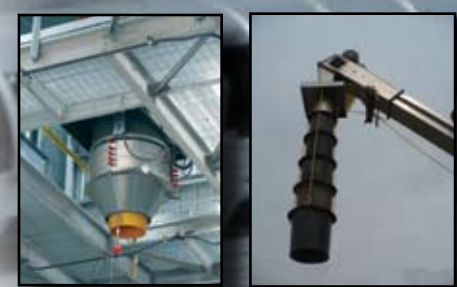
(L) Motorized dust control spout (R) Simple telescoping spout with manual winch
